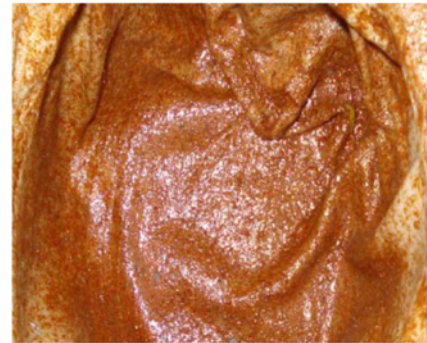
(5.b). Removed rust from the tank.
